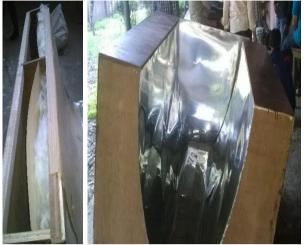
Fig.1 Parabolic domestic solar water heater
